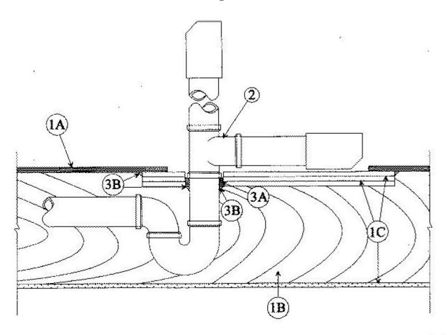
1. **Floor-Ceiling Assembly** — The fire-rated solid or trussed lumber joist floor-ceiling assembly shall be constructed of the materials and in the manner specified in individual L500 Series Floor-Ceiling Designs in the UL Fire Resistance Directory. The general construction details of the floor-ceiling assembly are summarized below:
