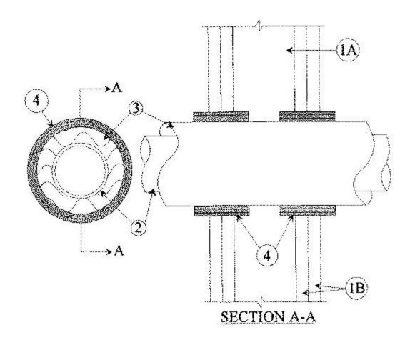
1. **Wall Assembly** — The fire-rated gypsum wallboard/stud wall assembly shall be constructed of the materials and in the manner specified in the individual U300 or U400 Series Wall and Partition Designs in the UL Fire Resistance Directory and shall include the following construction features:
