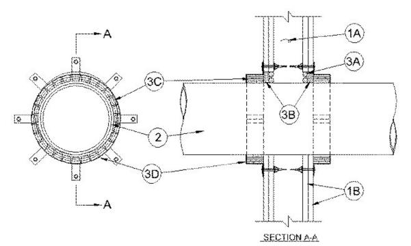
1. Wall Assembly — The 1 or 2 hr fire-rated gypsum board/stud wall assembly shall be constructed of the materials and in the manner specified in the individual U300, U400 or V400 Series Wall and Partition Designs in the UL Fire Resistance Directory and shall include the following construction features:
