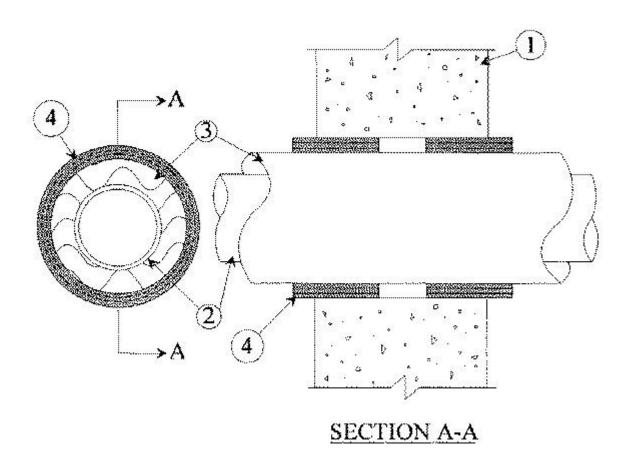
1. **Wall Assembly** — Min 5 in. thick reinforced lightweight or normal weight (100-150 pcf) concrete. Wall may also be constructed of any UL Classified **Concrete Blocks\*** having a minimum face shell thickness of 1-1/4 in. Max diam of opening is 18 in.
