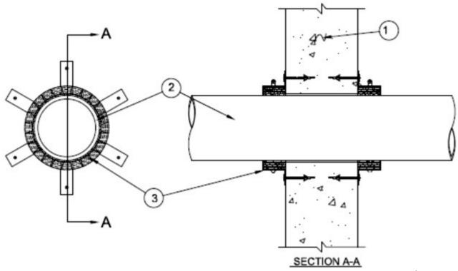
1. **Wall Assembly** — Min 6 in. (152 mm) thick lightweight or normal weight (100-150 pcf or 1600 - 2400 kg/m³) concrete. Wall may also be constructed of any UL Classified **Concrete Blocks\***. Max diam of opening is 5 in. (127 mm).
