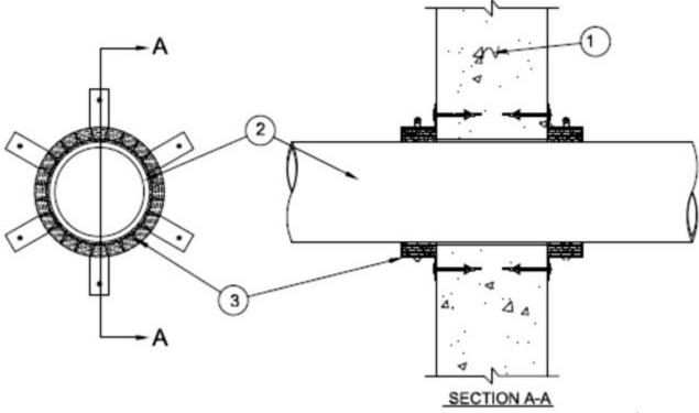
1. **Wall Assembly** — Min 6 in. (152 mm) thick lightweight or normal weight (100-150 pcf or 1600 - 2400 kg/m³) concrete. Wall may also be constructed of any UL Classified **Concrete Blocks\***. Max diam of opening is 5 in. (127 mm).
