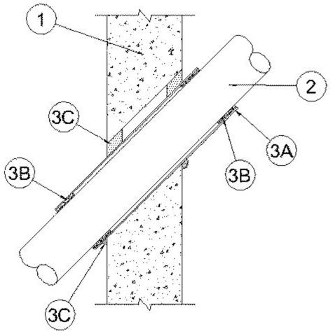
1. **Wall Assembly** — Min 6 in. thick reinforced lightweight or normal weight (100-150 pcf) concrete. Wall may also be constructed of any UL Classified **Concrete Blocks\***. Max diam of opening is 6 in.
