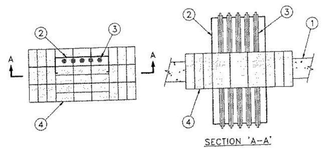
1. Floor or Wall Assembly — Min 4-1/2 in. thick reinforced lightweight (100 pcf) concrete. Max area of opening is 288 sq in. with max dimension of 24 in. Wall may also be constructed of any UL Classified Concrete Blocks\*.
