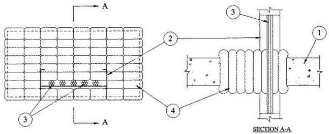
1. **Floor or Wall Assembly** — Min 5 in. thick reinforced normal weight (140-150 pcf) concrete. Wall may also be constructed of any UL Classified **Concrete Blocks\*.** Max area of opening is 288 sq in. with max dimensions of 24 in.
