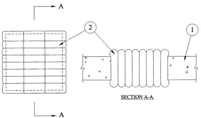
1. Floor or Wall Assembly — Min 5 in. thick reinforced normal weight (140-150 pcf) concrete. Wall may also be constructed of any UL Classified **Concrete Blocks\*.** Max area of opening is 144 sq in. with max dimensions of 12 in.
