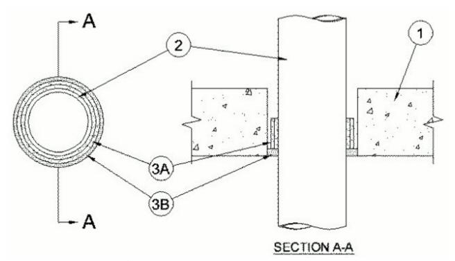
1. **Floor or Wall Assembly** — Min 4-1/2 in. thick reinforced lightweight or normal weight (100-150 pcf) concrete floor or min 5 in. thick reinforced lightweight or normal weight (100-150 pcf) concrete wall. Wall may also be constructed of any UL Classified **Concrete Blocks\***. Max diam of opening shall be 6 in.
